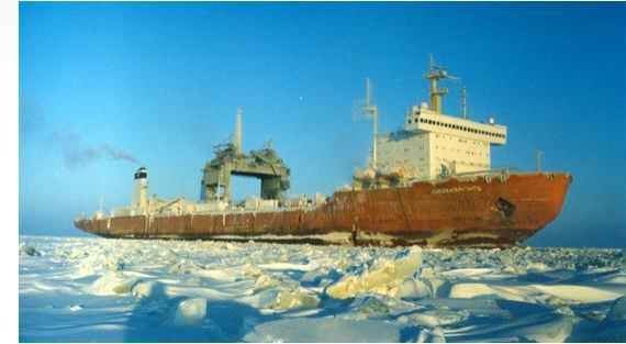
KLT-40 Russian Icebreaker Reactor (PWR, 35 MWe, basic design for floating nuclear power plant)
